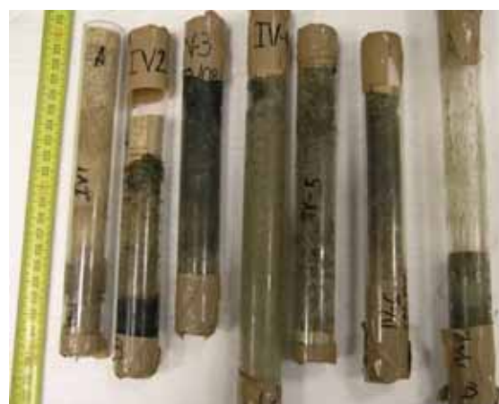
Figure 5-17 a) and b): Soil and clogging processes profiles collected in the stations for the study of clogging and infiltration capacity evolution for the stations IN (West channel) and IV (East channel). Their position is presented in Figure 5-18 cartography
