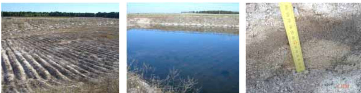
Figure 6-5 a) to c): Infiltration pond bench to test infiltration rate in order to different furrows wavelengths. The 80 cm distance has proved to be the most efficient for these environmental conditions
