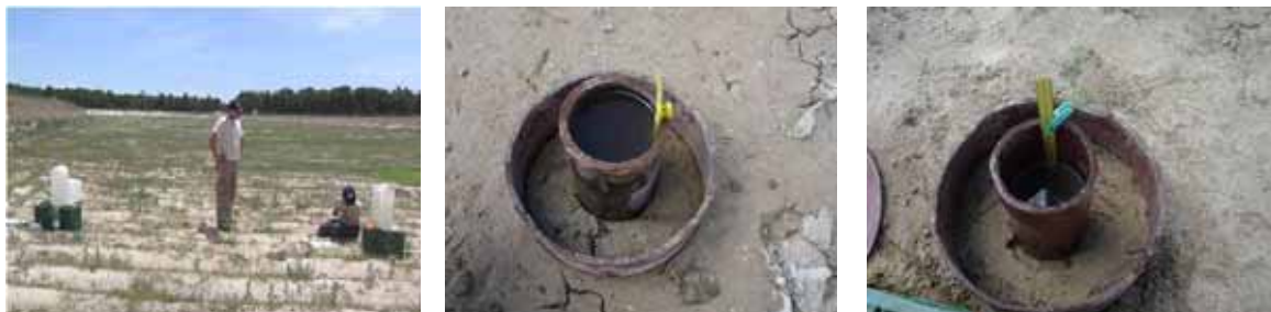
Figure 6-6 a) to c): Furrows plugged with different width at the bottom of a decantation and infiltration pond, infiltration test by double ring infiltrometer in the convex (sandy) and concave (clay) surface of them and the clogging profile. Headwater of the Santiuste's MAR device
