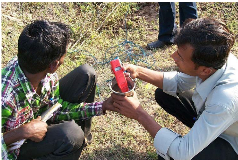
Fig. 4 Training BJs in the field— measuring groundwater quality
